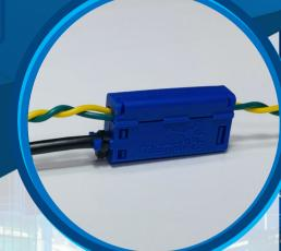
Qreader is a non- interfering and non-intrusive contactless CANbus data reader. It can collect CANbus data from all vehicle CANbus's. With Qreader, there is no need to strip wires and make a wire-to-wire soldering connections to read CANbus because herewith CANbus data is read over the isolation of the wire.
